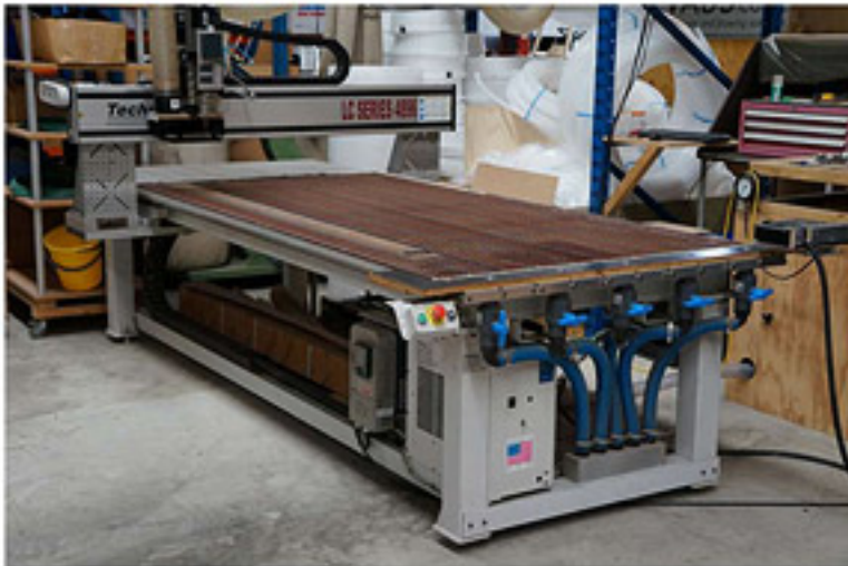
Techno 4896 - 7kW manual collet spindle
